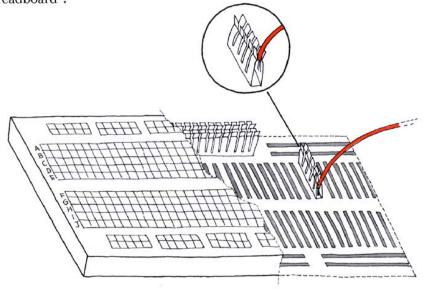
It is a small plastic board full of holes, each one of them containing a springloaded contact. When you push a component's leg into one of theses holes it establishes an electrical connection with all the other holes in the same vertical column. Each hole is at a distance of 2.54 mm from the others, since most of the components have their legs, (also known as pins) spaced at that standard distance. This is very practical for chips with multiple legs.
