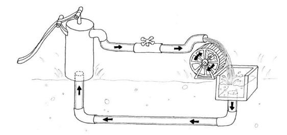
In this simple system two parameters are important: the pressure of the water (determined by how powerful the pump is) and the amount of water that can flow in the pipes (determined by the size of the pipes and the resistance that the wheel will oppose to the stream of water hitting it).
