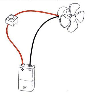
If you were to take it apart, you'll see that it contains a small battery, a few wires going to an electric motor one of which is interrupted by a switch. Make sure you have a new battery fitted into the device and activate the switch; the motor starts to spin.
