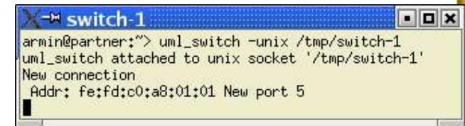
If you want to attach the UML host to the virtual switch your need root-access to configure a tap-device:
