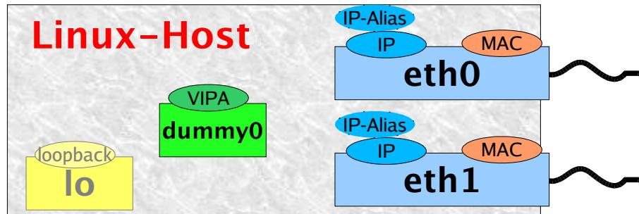
(Linux does not distinguish between Network- „Adapter“ and „Interface“)
